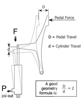
When a brake system is unable to hold the aircraft back at full static engine run-up, it is often the fault of the brake pedal geometry not exerting adequate force on the brake master cylinder.
