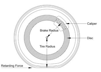
The moment about the axle of the brake must be equal to that of the tire which means that the retarding force on the tire ( $F_T$ ) times the rolling radius of the tire ( $R_T$ ) must be equal to the retarding force of the brake ( $F_B$ ) times the effective brake radius ( $R_B$ ).
