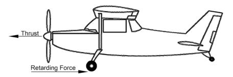
Simply put, the brake system must provide adequate torque on the wheel(s) to accomplish this. Several factors contribute to this — the brake pedal geometry, master cylinder piston diameter, brake caliper piston diameter, effective radius of the brake disc and the rolling radius of the tire.
