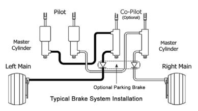
It is critically important that the installation allows the brake cylinder piston rod to fully extend when no load is applied.
