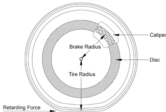
The moment about the axle of the brake must be equal to that of the tire which means that the retarding force on the tire ( $F_T$ ) times the rolling radius of the tire ( $R_T$ ) must be equal to the retarding force of the brake ( $F_B$ ) times the effective brake radius ( $R_B$ ).
