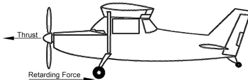
Simply put, the brake system must provide adequate torque on the wheel(s) to accomplish this. Several factors contribute to this — the brake pedal geometry, master cylinder piston diameter, brake caliper piston diameter, effective radius of the brake disc and the rolling radius of the tire.
