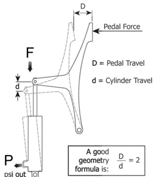
When a brake system is unable to hold the aircraft back at full static engine run-up, it is often the fault of the brake pedal geometry not exerting adequate force on the brake master cylinder.
