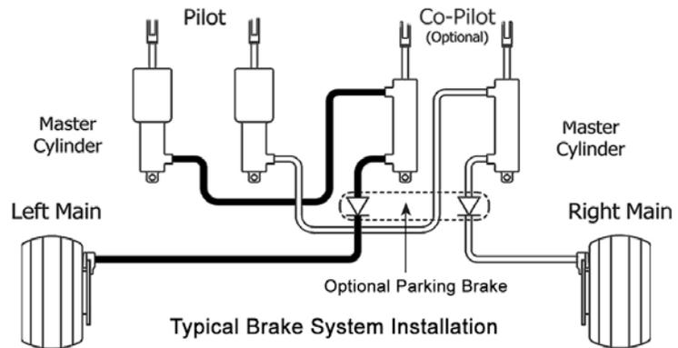
It is critically important that the installation allows the brake cylinder piston rod to fully extend when no load is applied.
